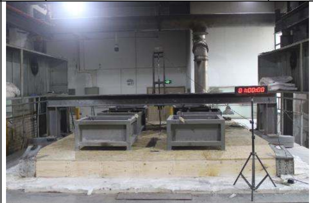
Photo 28: The unexposed face of sample (After test)
