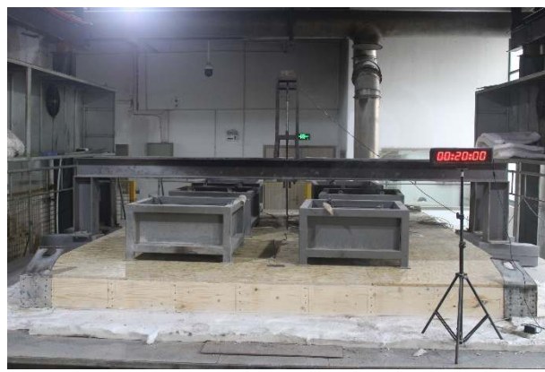
Photo 23: The unexposed face of sample (After test duration of 20 minutes)
