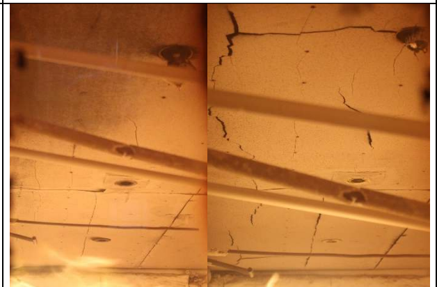
Photo 22: The exposed face of sample (After test duration of 5 & 20 minutes)
