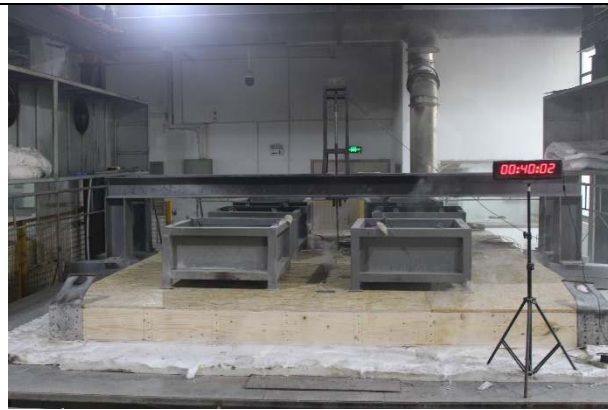
Photo 25: The unexposed face of sample (After test duration of 40 minutes)
