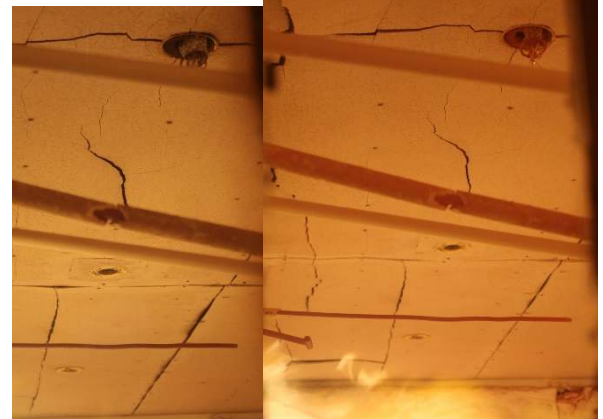
Photo 24: The exposed face of sample (After test duration of 30 & 40 minutes)
