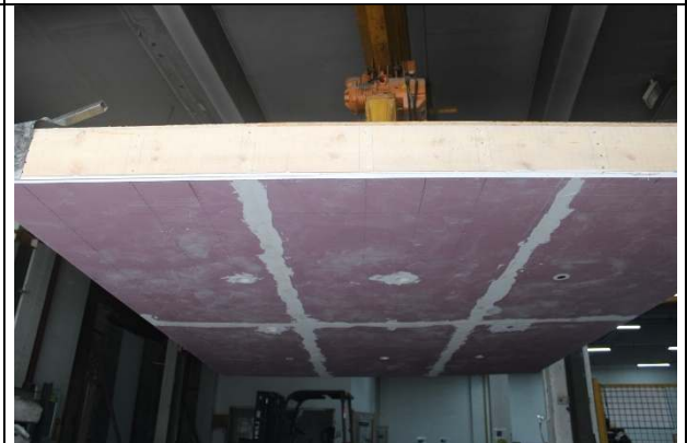
Photo 20: The exposed face before the test
