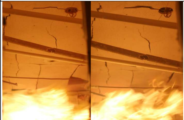
Photo 26: The exposed face of sample (After test duration of 50 & 55 minutes)
