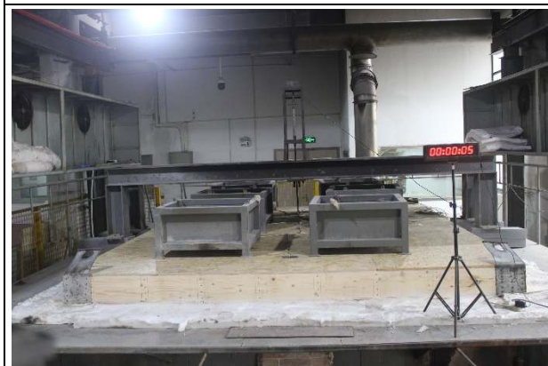
Photo 21: The unexposed face of sample (Test start)
