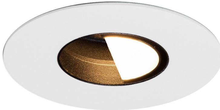
92mm (3.62") overall diameter. Shallow Height Low Output downlight. Edge baffle to ensure aperture is glare free and for a professional look. Available with standard trim kit or plaster-in kit for flush appearance. Family of matching products also available. Required depth height + 25mm^
